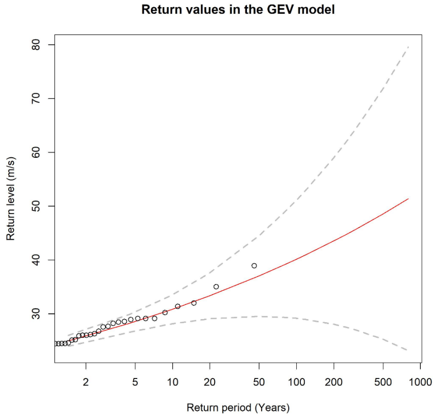
Figure 3-11 Return values of wind speed (m/s) at 100 m above sea level in the GEV model. Red curve represents the best fit with the data and aligns with the input data. Dashed lines represent the 95 % confidence intervals. Distribution parameters: location = 24.0669; scale = 2.6934; shape = 0.0819.
